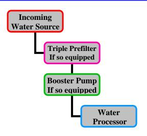
The Triple PreFilter is always installed closest to the source water. The Booster Pump goes before the processor and after the PreFilter if so equipped. Direction of FLOW is marked on both the Triple PreFilter and the Booster Pump. Point FLOW ARROWS towards the processor.
