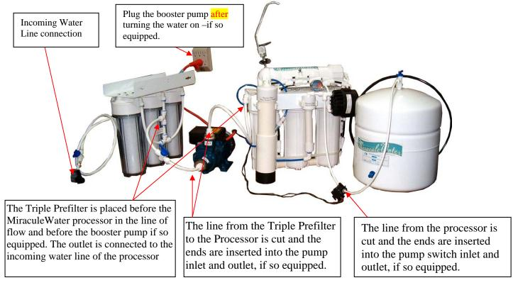
Firmly insert tubing when making these connections. To prevent leaks insure that the tubing is free of scratches before inserting into any fitting. Always insert tubing straight into the fitting and completely [about ½ inch]. Trim excess tubing as needed for best performance of the processor. Follow common sense flow pattern of connecting inlets and outlets as needed for your installation.
